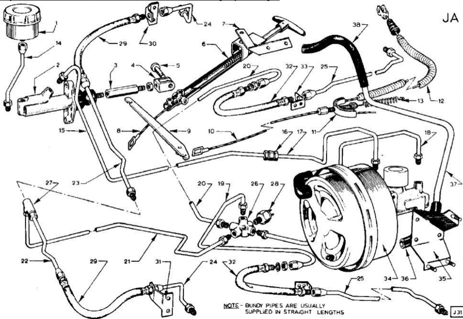
Lotus Europa TC/TCS Parts Manual - Section JA - Brakes - Handbrake and Single System - Page 2
