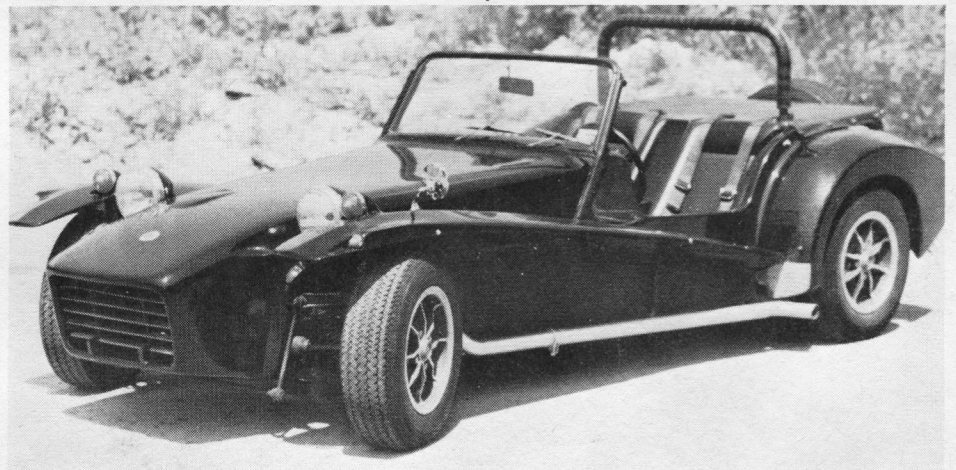
1972 Lotus Super 7 twin-cam with Checkpoint America turbo kit. Rajay 377B40 turbo pumps up to 21 psi. Single Stromberg CD 1-3/4 inch replaced dual twin-choke Webers. Boost starts at 1500 RPM and a rev limiter is set at 7000 RPM. Lucas distributor is used with a CD unit. Fuel consumption is 37 MPG.
