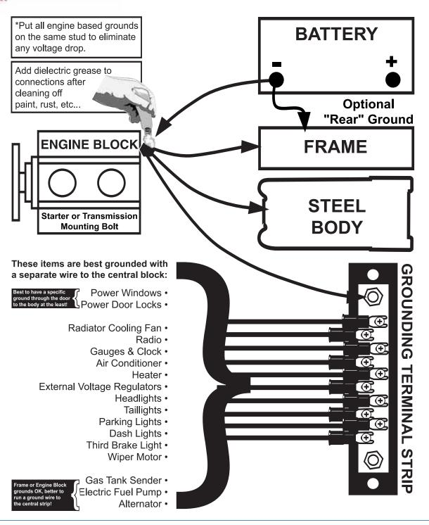
TIP# 106 Is it possible to have "too many grounds"? No, not the way too many fuses can cause a problem. Fuses have to be in series which means any one failure will shut it down. Grounds are in parallel and any failure only means one less good connection, but the others will carry it.
