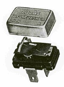
ribbon, the metal vane, and terminal L. Current flowing through the metal ribbon causes the latter to heat and expand, allowing the vane to relax and so to open the contacts. The signal lamp bulbs are now extinguished, the ribbon cools and re-tensions the vane, closing the contacts for the cycle to be repeated.
